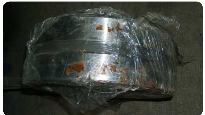
Fig. 3 Bearing, in storage, corroded by humidity.
