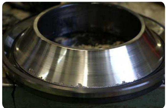
Fig. 2 Bearing made from upgraded steel with spalling
